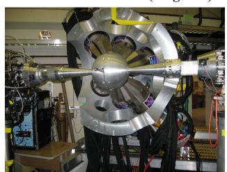
Charge breeder + upgraded ATLAS provides post-acceleration with ~10% total efficiency and exquisite beam properties
